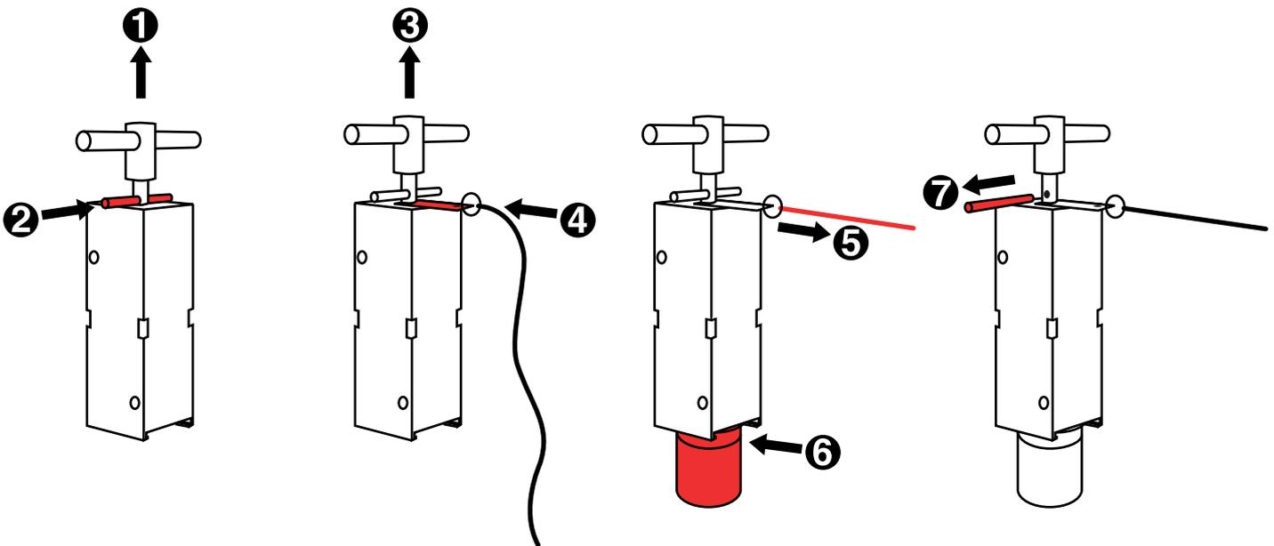
1. Pull up the firing pin until you can see the hole for inserting the safety device.
